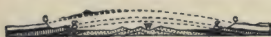
FIG. 84.—Section across the Weald from North to South. cc Chalk, gg Greensand escarpments, w Wealden sandstones.
